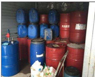
Photo of non-conformity No secondary container.JPG
