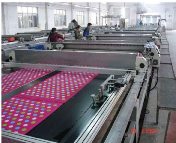
Printing lines: 5 lines 1. Make silk screen with your artwork 2. Printing on the machine 3. Fixed colors and processing
